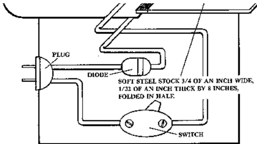
Figure 30. The magnetic pick is easy to construct.
