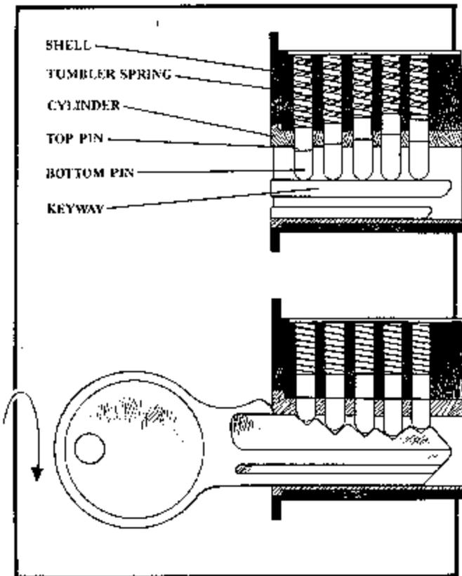
Figure 1. The pin tumbler lock, cutaway view.
