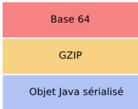
Fig 2: ViewState encoding without a security layer.
