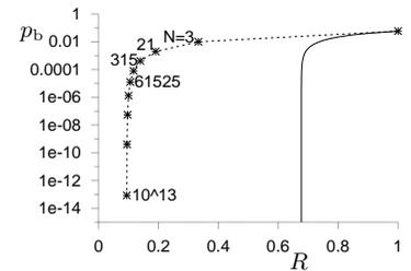
Figure 13.14. The bit error probabilities versus the rates  $R$  of the concatenated Hamming codes, for the binary symmetric channel with  $f = 0.0588$ . The solid line shows the Shannon limit for this channel.
