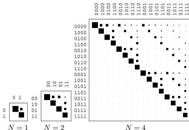
Figure 9.7. Extended channels obtained from a Z channel with transition probability 0.15. Each column corresponds to an input, and each row is a different output.
