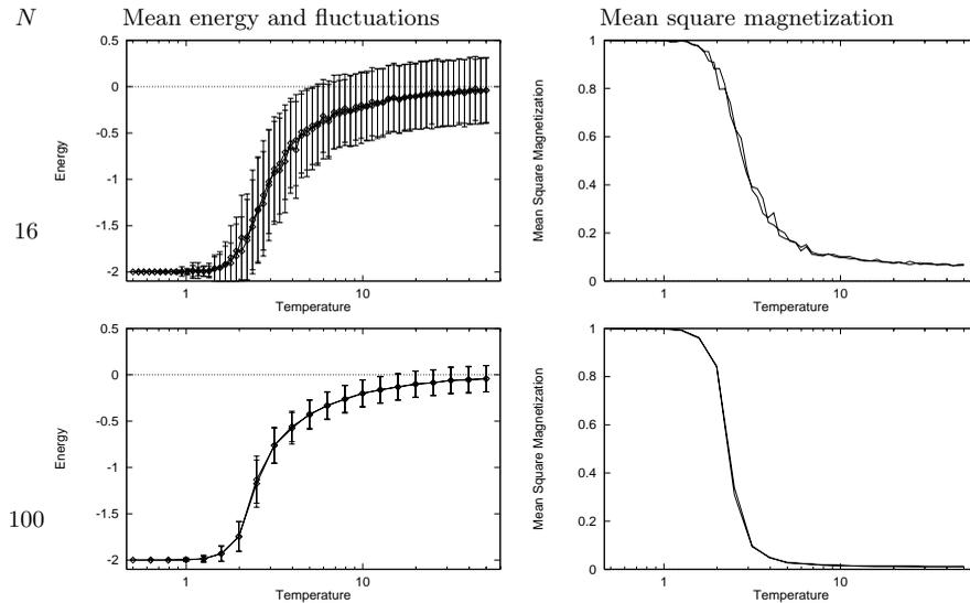
Figure 31.3. Monte Carlo simulations of rectangular Ising models with  $J = 1$ . Mean energy and fluctuations in energy as a function of temperature (left). Mean square magnetization as a function of temperature (right). In the top row,  $N = 16$ , and the bottom,  $N = 100$ . For even larger  $N$ , see later figures.
