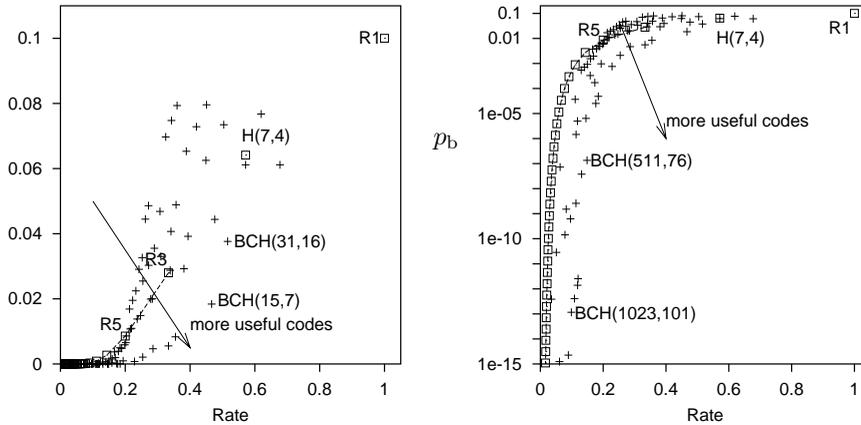
Figure 1.18. Error probability  $p_b$  versus rate  $R$  for repetition codes, the (7, 4) Hamming code and BCH codes with block lengths up to 1023 over a binary symmetric channel with  $f = 0.1$ . The righthand figure shows  $p_b$  on a logarithmic scale.
