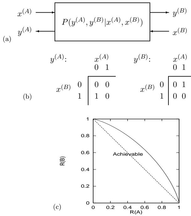
Figure 15.9. (a) A general two-way channel. (b) The rules for a binary two-way channel. The two tables show the outputs  $y^{(A)}$  and  $y^{(B)}$  that result for each state of the inputs. (c) Achievable region for the two-way binary channel. Rates below the solid line are achievable. The dotted line shows the ‘obviously achievable’ region which can be attained by simple time-sharing.
