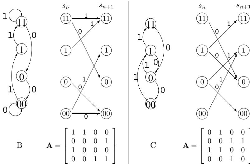
Figure 17.3. State diagrams, trellis sections and connection matrices for channels B and C.
