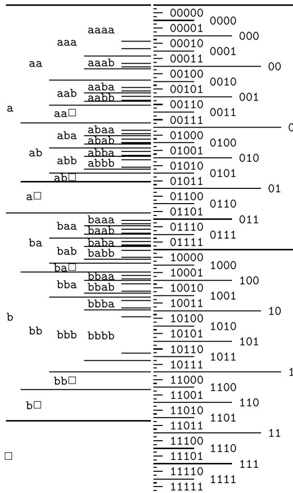
Figure 6.5. Illustration of the intervals defined by a simple Bayesian probabilistic model. The size of an intervals is proportional to the probability of the string. This model anticipates that the source is likely to be biased towards one of **a** and **b**, so sequences having lots of **a**s or lots of **b**s have larger intervals than sequences of the same length that are 50:50 **a**s and **b**s.
