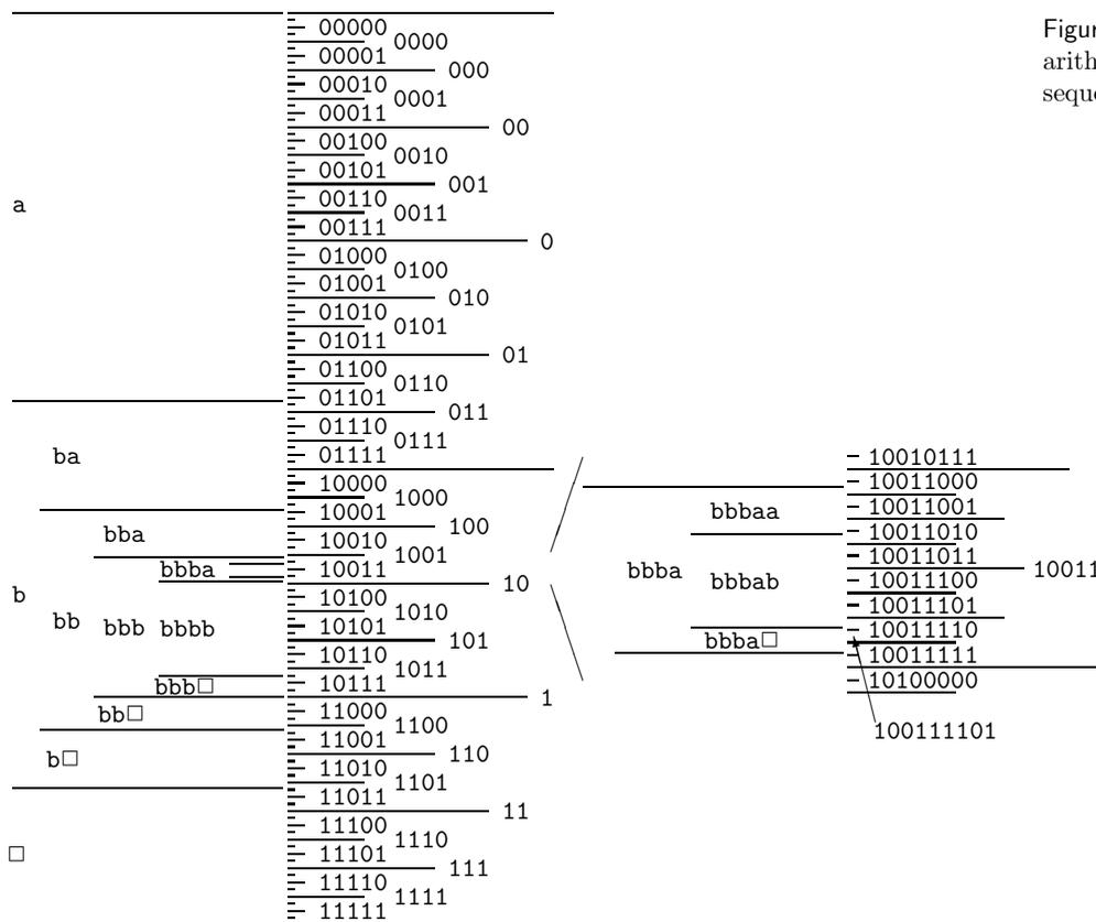
Figure 6.4. Illustration of the arithmetic coding process as the sequence **bbba** $\square$  is transmitted.
