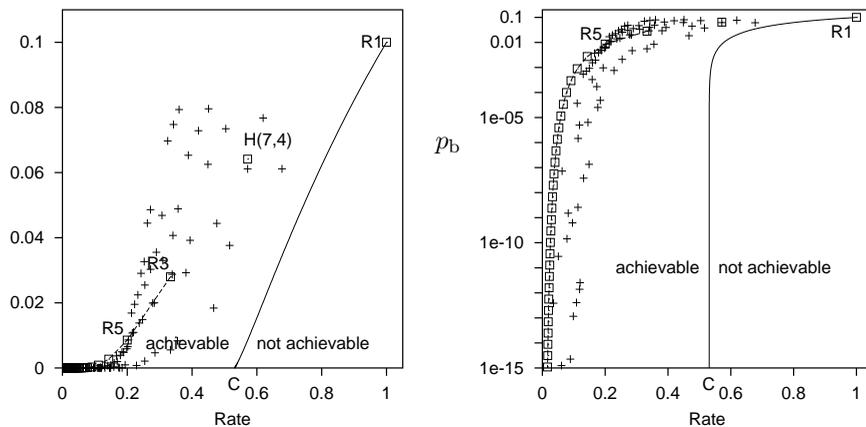
Figure 1.19. Shannon's noisy-channel coding theorem. The solid curve shows the Shannon limit on achievable values of  $(R, p_b)$  for the binary symmetric channel with  $f = 0.1$ . Rates up to  $R = C$  are achievable with arbitrarily small  $p_b$ . The points show the performance of some textbook codes, as in figure 1.18.
