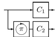
Figure 11.7. The encoder of a turbo code. Each box  $C_1$ ,  $C_2$ , contains a convolutional code. The source bits are reordered using a permutation  $\pi$  before they are fed to  $C_2$ . The transmitted codeword is obtained by concatenating or interleaving the outputs of the two convolutional codes. The random permutation is chosen when the code is designed, and fixed thereafter.
