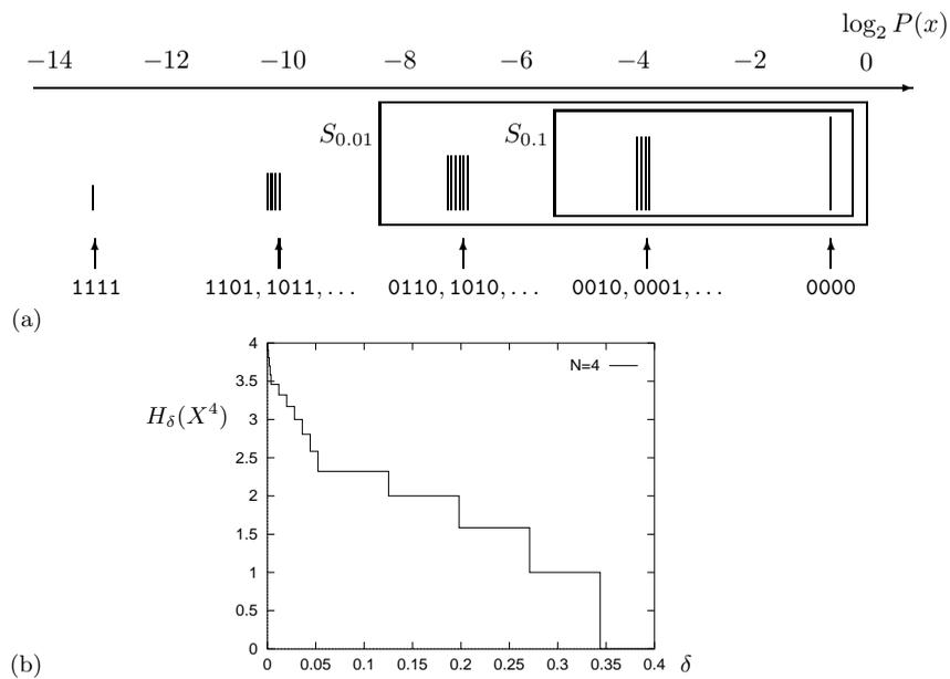
Figure 4.7. (a) The sixteen outcomes of the ensemble  $X^4$  with  $p_1 = 0.1$ , ranked by probability. (b) The essential bit content  $H_\delta(X^4)$ . The upper schematic diagram indicates the strings' probabilities by the vertical lines' lengths (not to scale).
