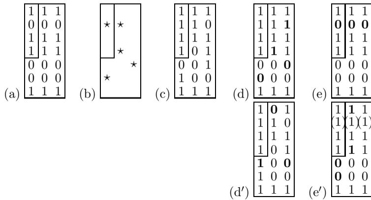
Figure 11.6. A product code. (a) A string 1011 encoded using a concatenated code consisting of two Hamming codes,  $H(3, 1)$  and  $H(7, 4)$ . (b) a noise pattern that flips 5 bits. (c) The received vector. (d) After decoding using the horizontal  $(3, 1)$  decoder, and (e) after subsequently using the vertical  $(7, 4)$  decoder. The decoded vector matches the original. (d', e') After decoding in the other order, three errors still remain.
