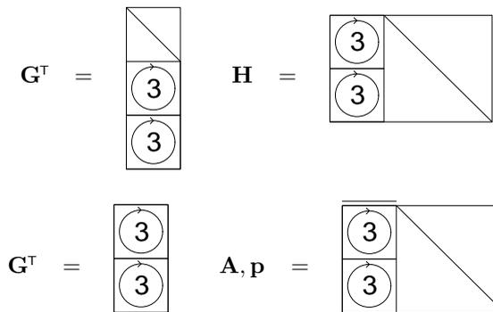
Figure 49.5. The generator matrix and parity-check matrix of a systematic low-density generator-matrix code. The code has rate  $1/3$ .
