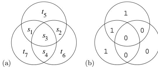
Figure 1.13. Pictorial representation of encoding for the (7, 4) Hamming code.
