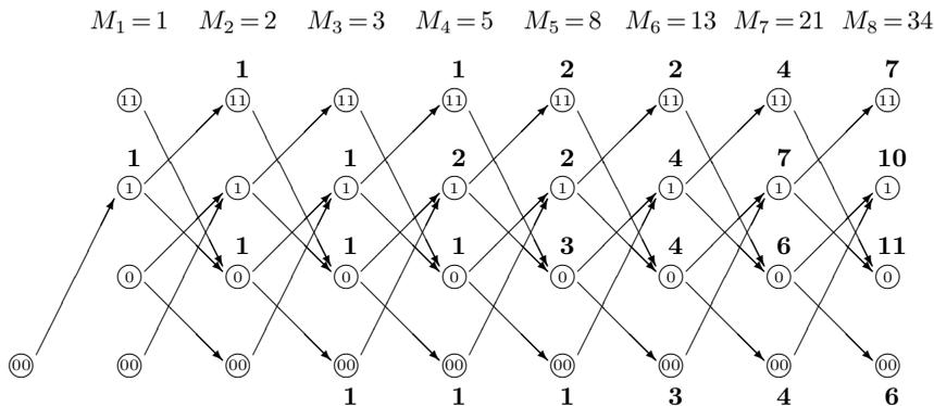
Figure 17.5. Counting the number of paths in the trellises of channels A, B, and C. We assume that at the start the first bit is preceded by 00, so that for channels A and B, any initial character is permitted, but for channel C, the first character must be a 1.
