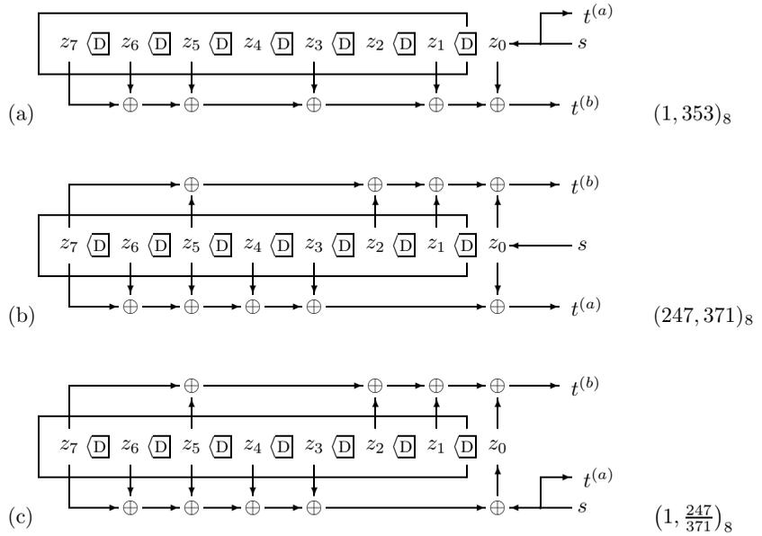
Figure 48.1. Linear feedback shift registers for generating convolutional codes with rate 1/2. The symbol  $\langle \text{D} \rangle$  indicates a copying with a delay of one clock cycle. The symbol  $\oplus$  denotes linear addition modulo 2 with no delay.
