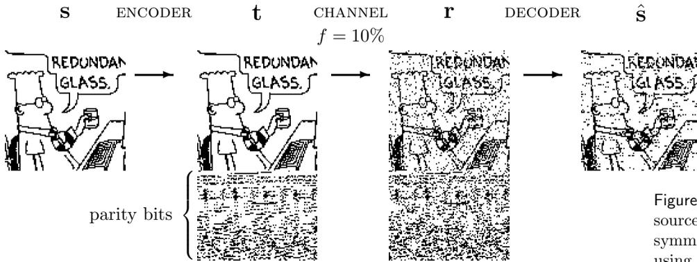
Figure 1.17. Transmitting 10 000 source bits over a binary symmetric channel with  $f = 10\%$  using a  $(7, 4)$  Hamming code. The probability of decoded bit error is about 7%.
