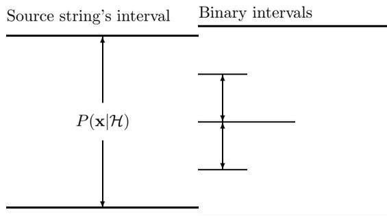
Figure 6.10. Termination of arithmetic coding in the worst case, where there is a two bit overhead. Either of the two binary intervals marked on the right-hand side may be chosen. These binary intervals are no smaller than  $P(\mathbf{x}|\mathcal{H})/4$ .
