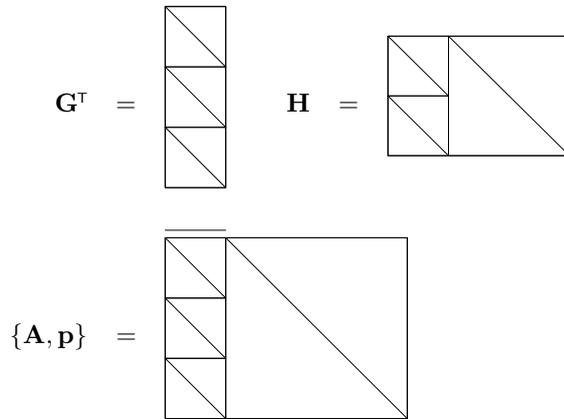
Figure 49.4. The generator matrix, parity-check matrix, and a generalized parity-check matrix of a repetition code with rate  $1/3$ .
