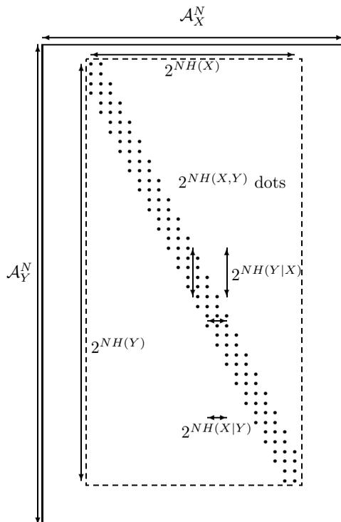
Figure 10.2. The jointly typical set. The horizontal direction represents  $\mathcal{A}_X^N$ , the set of all input strings of length  $N$ . The vertical direction represents  $\mathcal{A}_Y^N$ , the set of all output strings of length  $N$ . The outer box contains all conceivable input–output pairs. Each dot represents a jointly typical pair of sequences  $(\mathbf{x}, \mathbf{y})$ . The total number of jointly typical sequences is about  $2^{NH(X,Y)}$ .
