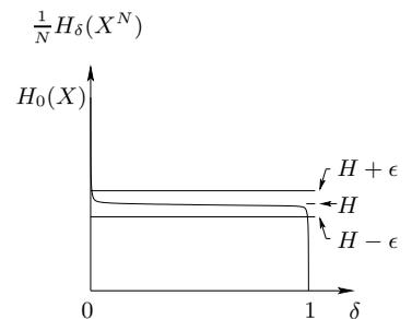
Figure 4.13. Schematic illustration of the two parts of the theorem. Given any  $\delta$  and  $\epsilon$ , we show that for large enough  $N$ ,  $\frac{1}{N} H_\delta(X^N)$  lies (1) below the line  $H + \epsilon$  and (2) above the line  $H - \epsilon$ .
