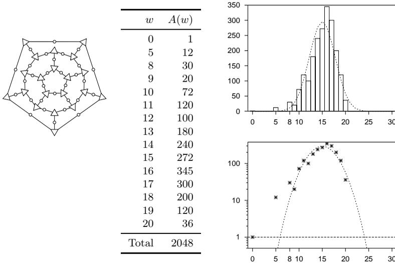
Figure 13.2. The graph defining the (30, 11) dodecahedron code (the circles are the 30 transmitted bits and the triangles are the 20 parity checks, one of which is redundant) and the weight enumerator function (solid lines). The dotted lines show the average weight enumerator function of all random linear codes with the same size of generator matrix, which will be computed shortly. The lower figure shows the same functions on a log scale.
