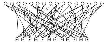
Figure 1.22. Graph of a rate- $1/4$  low-density parity-check code (Gallager code) with blocklength  $N = 16$ , and  $M = 12$  parity-check constraints. Each white circle represents a transmitted bit. Each bit participates in  $j = 3$  constraints, represented by  $\square$  squares. The edges between nodes were placed at random. (See Chapter 47 for more.)
