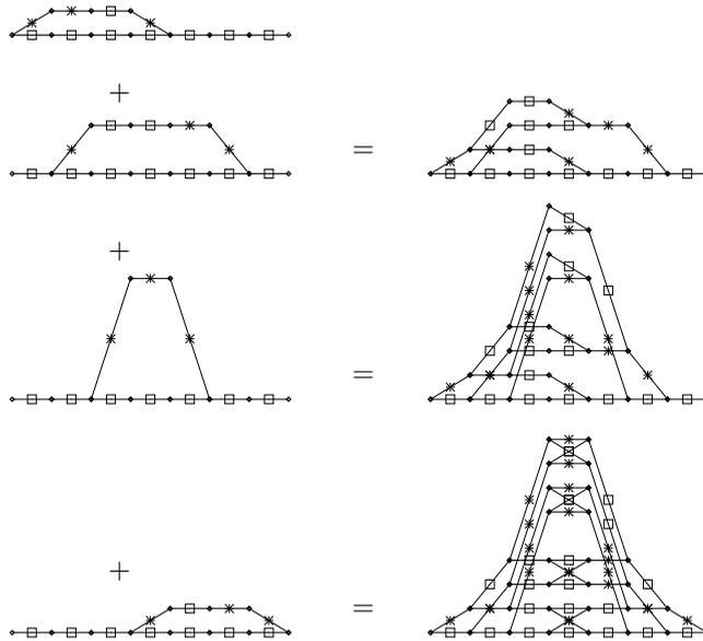
Figure 25.6. Trellises for four subcodes of the (7, 4) Hamming code (left column), and the sequence of trellises that are made when constructing the trellis for the (7, 4) Hamming code (right column).
