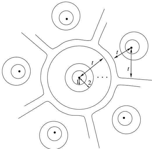
Figure 13.4. Schematic picture of part of Hamming space perfectly filled by  $t$ -spheres centred on the codewords of a perfect code.
