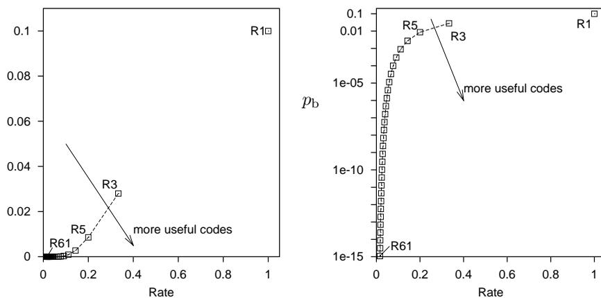
Figure 1.12. Error probability  $p_b$  versus rate for repetition codes over a binary symmetric channel with  $f = 0.1$ . The right-hand figure shows  $p_b$  on a logarithmic scale. We would like the rate to be large and  $p_b$  to be small.
