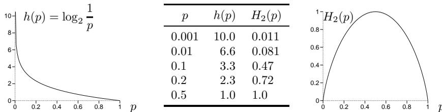
Figure 4.1. The Shannon information content  $h(p) = \log_2 \frac{1}{p}$  and the binary entropy function  $H_2(p) = H(p, 1-p) = p \log_2 \frac{1}{p} + (1-p) \log_2 \frac{1}{(1-p)}$  as a function of  $p$ .
