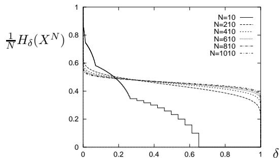
Figure 4.9.  $\frac{1}{N} H_\delta(X^N)$  for  $N = 10, 210, \dots, 1010$  binary variables with  $p_1 = 0.1$ .
