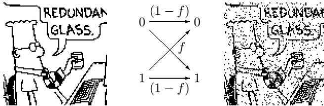
Figure 1.5. A binary data sequence of length 10 000 transmitted over a binary symmetric channel with noise level  $f = 0.1$ . [Dilbert image Copyright©1997 United Feature Syndicate, Inc., used with permission.]
