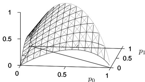
**Special cases.** In the special case  $p_? = 0$ , the channel is a noiseless binary channel, and  $I(X; Y) = H_2(p_0)$ .
