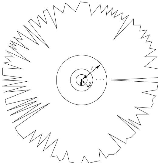
Figure 13.11. Berlekamp's schematic picture of Hamming space in the vicinity of a codeword. The jagged solid line encloses all points to which this codeword is the closest. The  $t$ -sphere around the codeword takes up a small fraction of this space.
