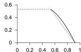
Figure 15.8. An achievable region for the channel with unknown noise level. Assuming the two possible noise levels are  $f_A = 0.01$  and  $f_B = 0.1$ , the dashed lines show the rates  $R_A, R_B$  that are achievable using a simple time-sharing approach, and the solid line shows rates achievable using a more cunning approach.
