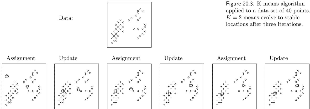
Figure 20.3. K means algorithm applied to a data set of 40 points.  $K = 2$  means evolve to stable locations after three iterations.
