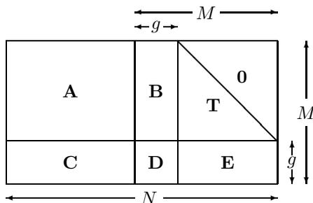
Figure 47.19. The parity-check matrix in approximate lower-triangular form.
