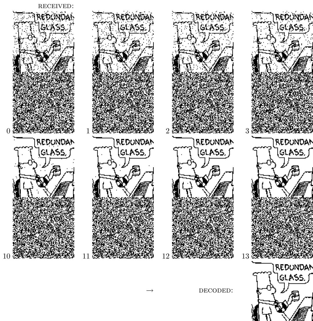
Figure 47.5. Iterative probabilistic decoding of a low-density parity-check code for a transmission received over a channel with noise level  $f = 7.5\%$ . The sequence of figures shows the best guess, bit by bit, given by the iterative decoder, after 0, 1, 2, 3, 10, 11, 12, 13 iterations. The decoder halts after the 13th iteration when the best guess violates no parity checks. This final decoding is error free.
