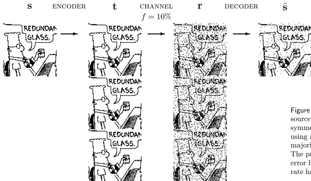
Figure 1.11. Transmitting 10 000 source bits over a binary symmetric channel with  $f = 10\%$  using a repetition code and the majority vote decoding algorithm. The probability of decoded bit error has fallen to about 3%; the rate has fallen to  $1/3$ .
