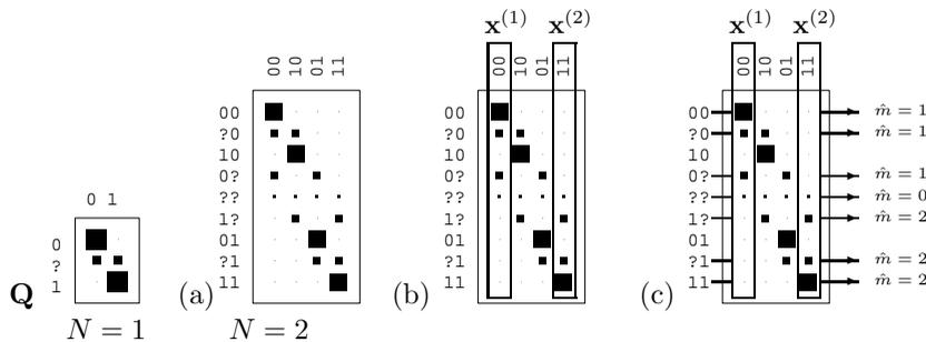
Figure 9.10. (a) The extended channel ( $N = 2$ ) obtained from a binary erasure channel with erasure probability 0.15. (b) A block code consisting of the two codewords 00 and 11. (c) The optimal decoder for this code.
