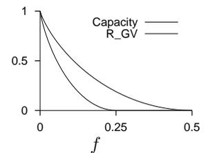
Figure 13.9. Contrast between Shannon’s channel capacity  $C$  and the Gilbert rate  $R_{GV}$  – the minimum communication rate achievable using a bounded-distance decoder, as a function of noise level  $f$ . For any given rate,  $R$ , the minimum tolerable noise level for Shannon is twice as big as the minimum tolerable noise level for a ‘worst-case-ist’ who uses a bounded-distance decoder.
