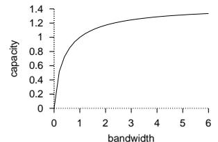
Figure 11.5. Capacity versus bandwidth for a real channel:  $C/W_0 = W/W_0 \log(1 + W_0/W)$  as a function of  $W/W_0$ .
