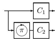
Figure 48.10. The encoder of a turbo code. Each box  $C_1, C_2$ , contains a convolutional code. The source bits are reordered using a permutation  $\pi$  before they are fed to  $C_2$ . The transmitted codeword is obtained by concatenating or interleaving the outputs of the two convolutional codes.
