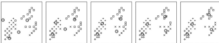
Figure 20.4. K means algorithm applied to a data set of 40 points. Two separate runs, both with  $K = 4$  means, reach different solutions. Each frame shows a successive assignment step.
