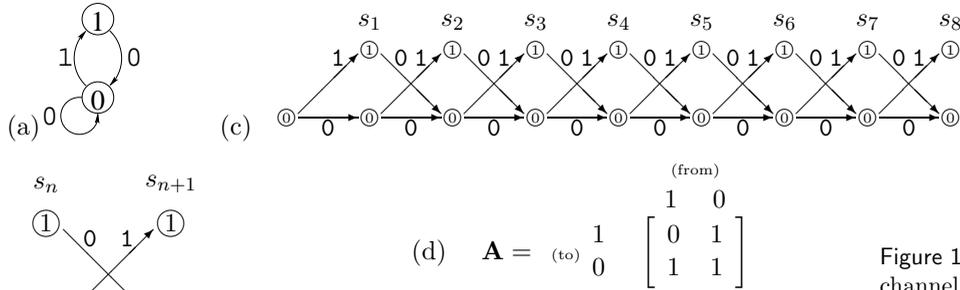
Figure 17.2. (a) State diagram for channel A. (b) Trellis section. (c) Trellis. (d) Connection matrix.
