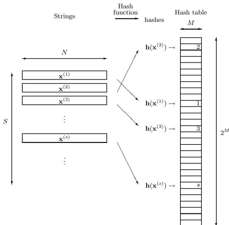
Figure 12.4. Use of hash functions for information retrieval. For each string  $x^{(s)}$ , the hash  $h = h(x^{(s)})$  is computed, and the value of  $s$  is written into the  $h$ th row of the hash table. Blank rows in the hash table contain the value zero. The table size is  $T = 2^M$ .
