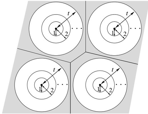
Figure 13.5. Schematic picture of Hamming space not perfectly filled by  $t$ -spheres centred on the codewords of a code. The grey regions show points that are at a Hamming distance of more than  $t$  from any codeword. This is a misleading picture, as, for any code with large  $t$  in high dimensions, the grey space between the spheres takes up almost all of Hamming space.
