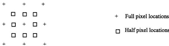
**FIGURE 16.3** Half-pixel locations in motion compensation.
