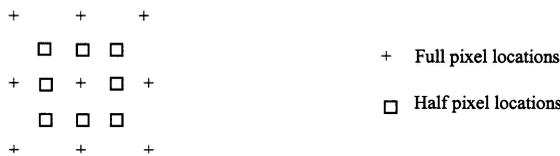
**FIGURE 16.3** Half-pixel locations in motion compensation.
