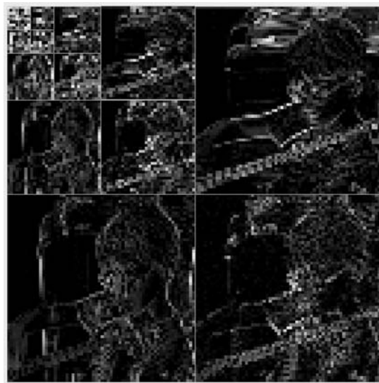
Figure 3.35 Five-stage wavelet decomposition of image
