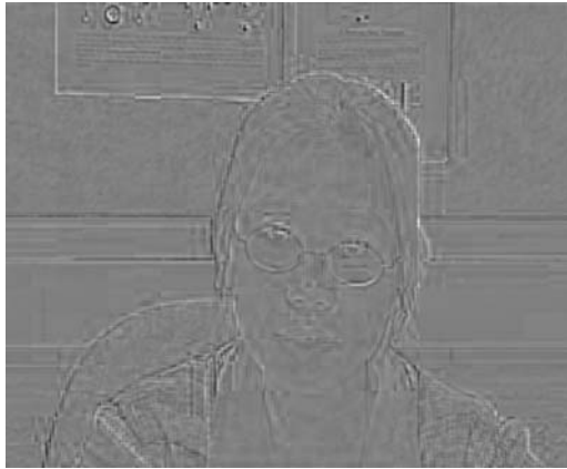
Figure 5.61 Residual to be encoded as enhancement layer
