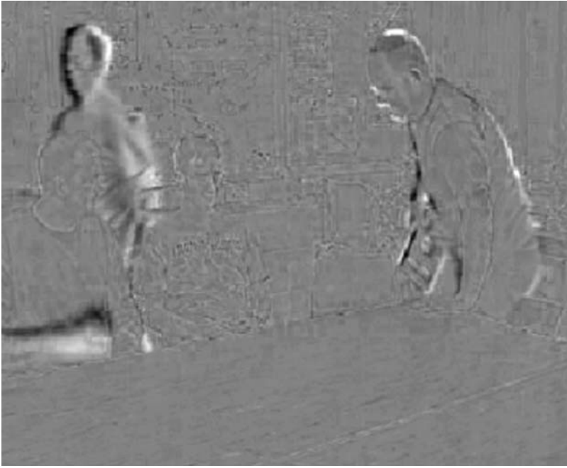
Figure 3.54 Residual F_n - F'_{n-1} (no motion compensation)
