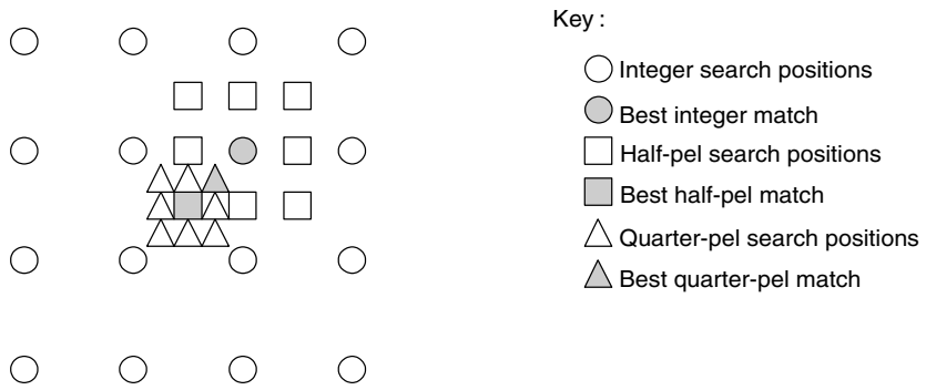
Figure 3.18 Integer, half-pixel and quarter-pixel motion estimation
