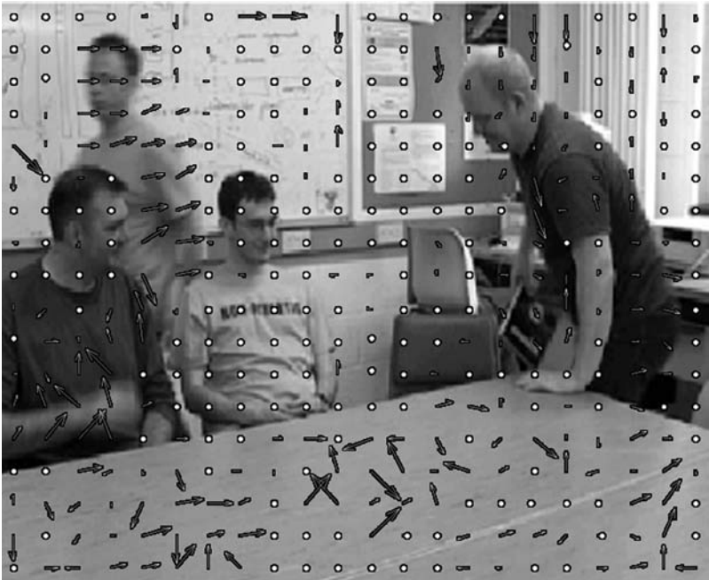
Figure 3.55 16 \times 16 motion vectors (superimposed on frame)
