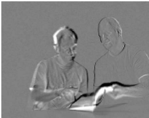
Figure 3.12 Residual (no motion compensation)
