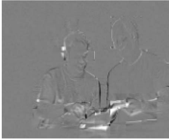
Figure 3.13 Residual ( 16 \times 16 block size)
