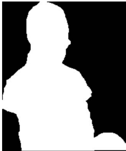
Figure 5.31 Binary alpha mask (complete VOP)
