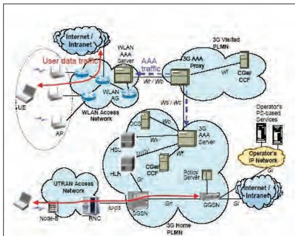
Figure 3. Wireless LAN/3G interworking architecture for Scenario 3
