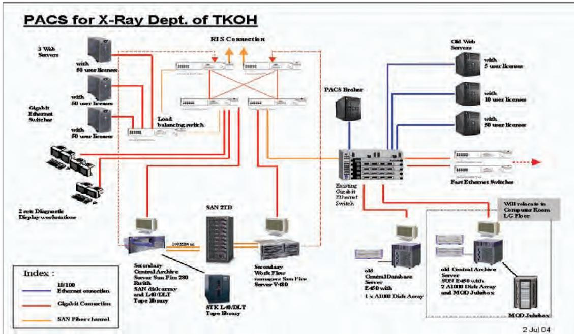
Figure 3. Design of a PACS and hospital network interface
