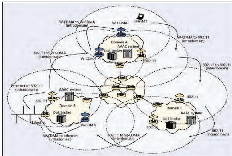
UMTS/WLAN environment in a single operator's network, the hierarchical policy architecture is used, as shown in Figure 5. The master policy controller (MPDF) connects to the policy controller of the wireless LAN network (WPDF) and the UMTS policy controller (PDF). The MPDF of the UMTS network serves as the master policy node of the WPDF so that the policies implemented in the wireless LAN domain are integrated into the operator's policy hierarchy.
