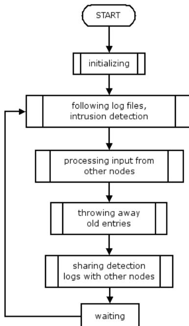
Figure 4 presents the algorithm of the software Komondor. It checks the log files every second, while the database should be purged only on hourly or on a daily basis (Czirkos, 2005).
