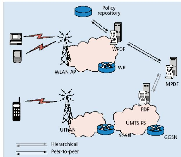
in this environment, a WPDF is deployed in the shared wireless LAN domain. As shown in Figure 6, the WPDF interacts with the MPDFs of the cooperating operators' networks.
