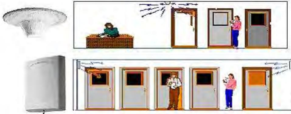
place the antenna in the corner of a corridor, providing coverage in a certain floor towards a certain direction (using of course directional in-door antenna). Figure 5 provides the omnidirectional and directional antenna types, while Figure 6 provides the indoor coverage based on these antenna.
