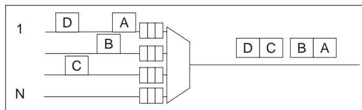
Figure 3. Connection-oriented packet switching
