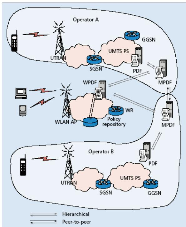
Figure 7. Customers' wireless LAN connected to an operator's UMTS
