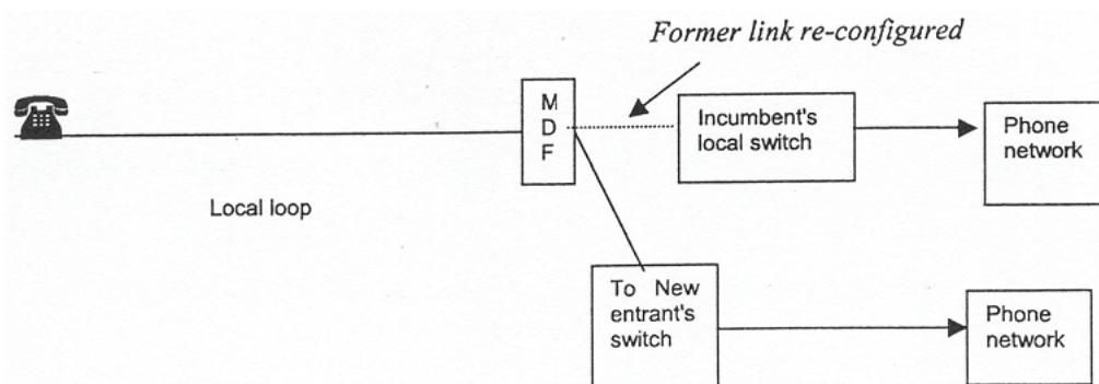
Figure 1(b). Case of “full” LLU, via the use of xDSL modem
