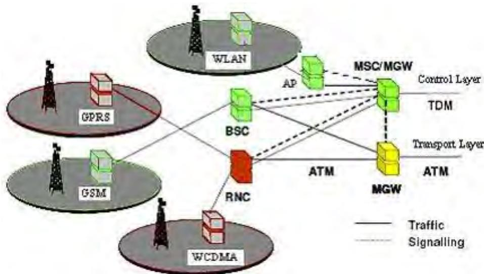
Figure 4. The different paths of voice and packet connections
