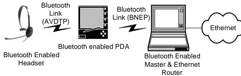
Figure 4. Interface module design architecture for audio streaming and voice playback
