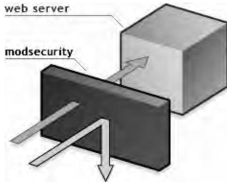
ModSecurity machine. After scanning the traffic, it can be forwarded to the appropriate Web server.
