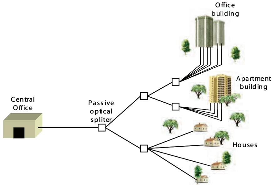
Figure 2. Schematic representation of a tree-and-branch topology for EPONs
