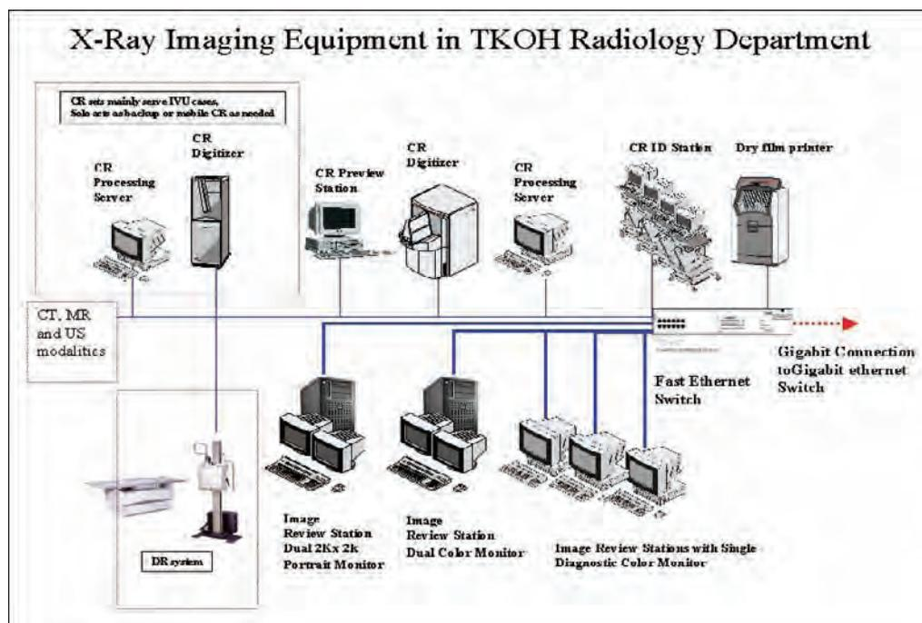
Figure 2. Design of the TKOH PACS
