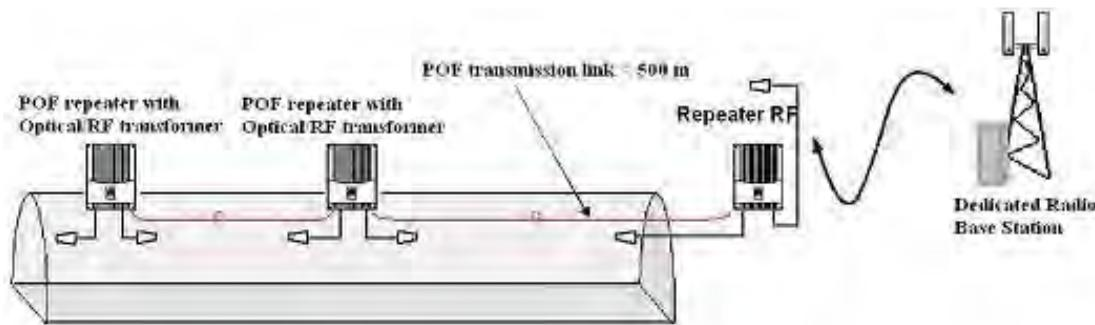
Figure 11. A combination method for tunnel coverage
