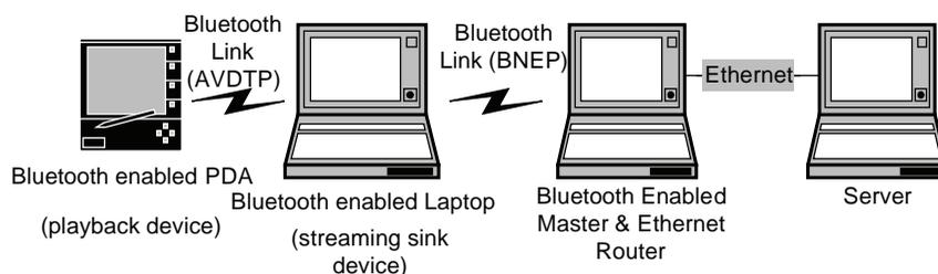
Figure 5. Experimental testbed with three Bluetooth devices and one Ethernet-based audio server
