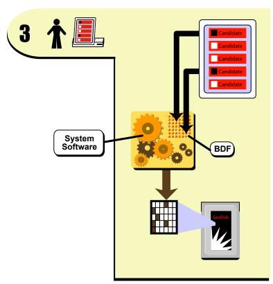
Figure 5: Casting a vote on the Diebold AccuVote TS
