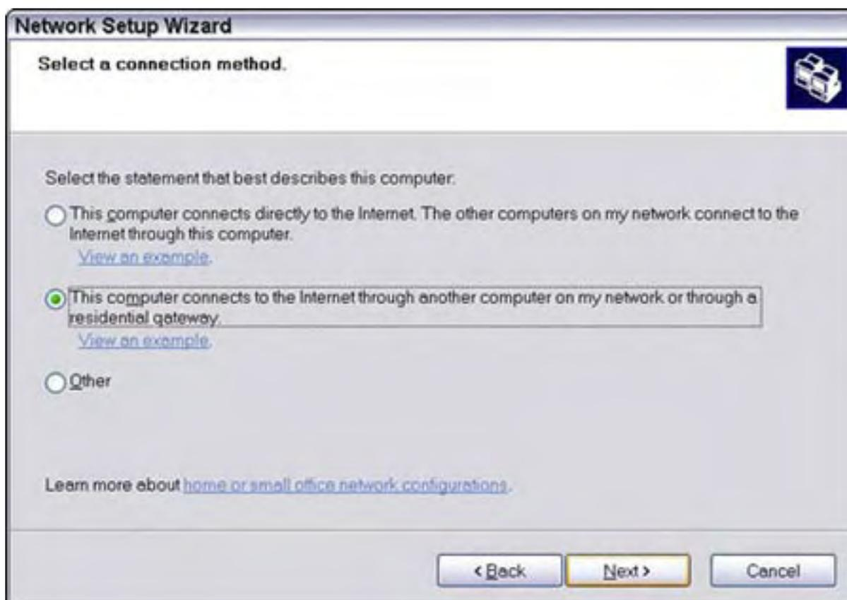
Figure 2-7: The Network Setup Wizard asking how you connect to the Internet.
