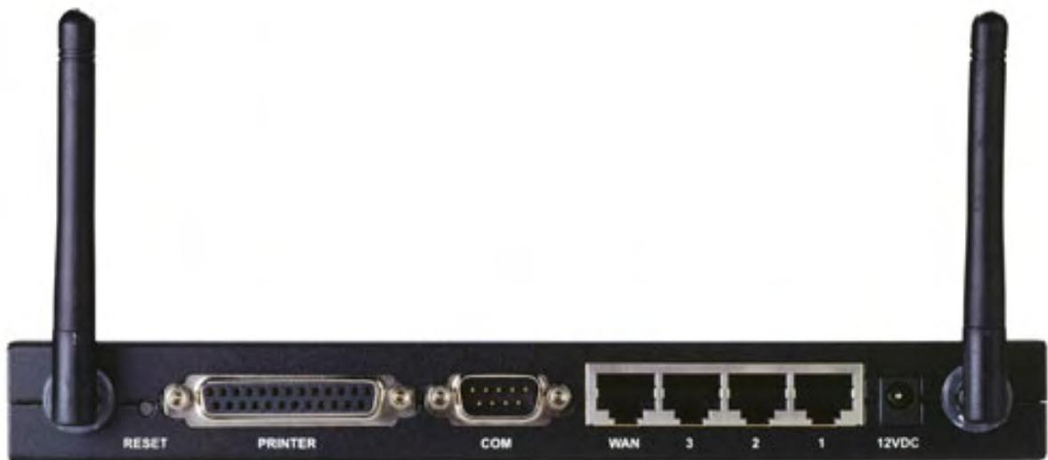
Figure 4-1: The printer connection on the back of a U.S. Robotics Model 8011 Wireless Cable and DSL Router.
