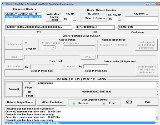
Fig. 10. ContactlessDemoVC.exe demo application from the OMNIKEY Synchronous API SDK - shows the successful read of data from inside the protected HID Access Control Application.
