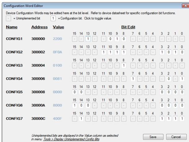
Fig. 5. Binary representation of the programming fuses
