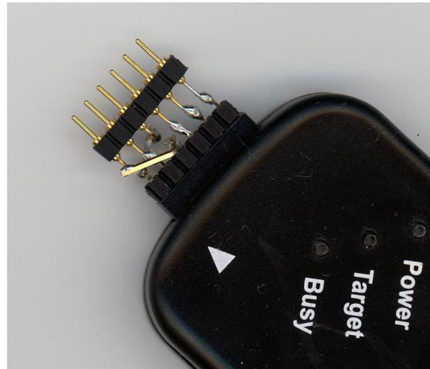
Fig. 3. Programming interface adapter for PICkit2 to switch Pin 1 with Pin 3.
