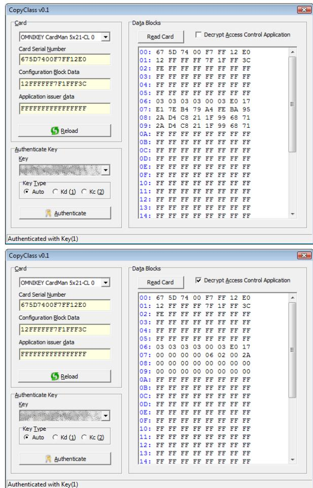
Fig. 11. CopyClass Tool v0.1 - encrypted & decrypted card content
