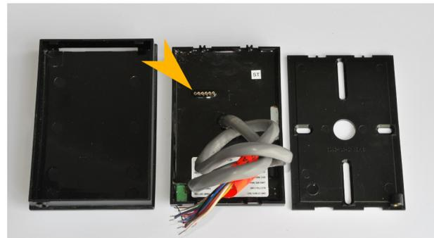
Fig. 2. RW400 programming interface. Pin 1 is top-left.
