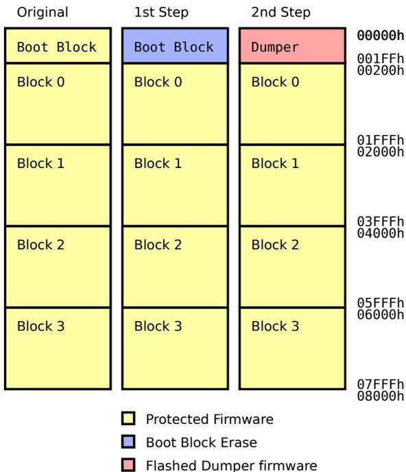
Fig. 6. In the first step EEPROM and FLASH content except of the boot block is dumped via UART.
