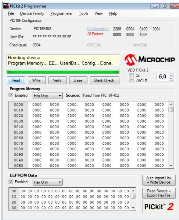
Fig. 4. PIC18F452 successfully detected - all copy protection and write protection fuses are set (“All Protect”) and code+EEPROM reads back all zeros as expected with copy protection set.
