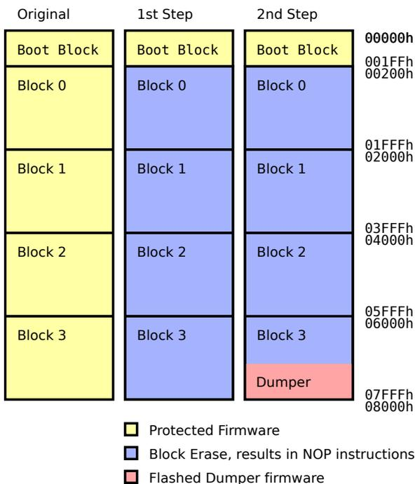
Fig. 7. In the second step the remaining bootblock is dumped via UART by putting the dumper code at the end of a trampoline of NOP instructions.
