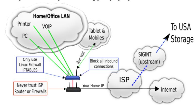
A second Linux firewall device (**blue**) that **you control and manage** is placed in front of the ISP router effectively placing the ISPs router in the Militarized Zone (MZ) i.e. the Internet. A single cable (**red**) is used to link the LAN of the ISP router to the Internet LAN port of the Linux firewall.
