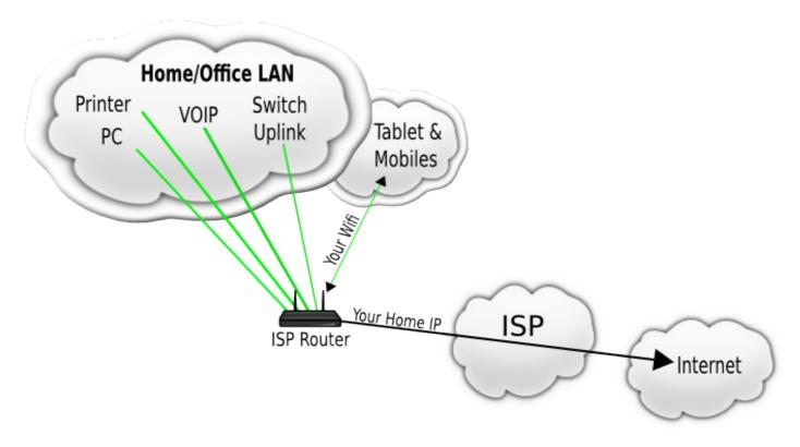
Most Internet connections consists of an DSL type modem and one or more Ethernet ports attached to the modem that you connect your computers, devices and add-on switches etc.
