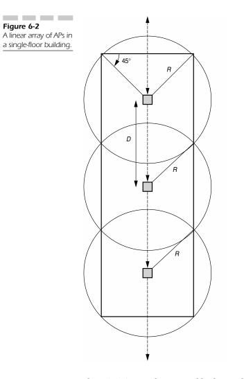
also minimizes as far as possible the overlap between and among AP coverage areas. A linear array is used when the building is narrow relative to R, and a rectangular array when the building width is large relative to R.
