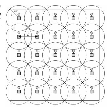
must dovetail with the coverage of the next AP's same floor coverage. As in a single-floor building, a linear array is used when the building is narrow relative to R, and a rectangular array when the building width is large relative to R.
