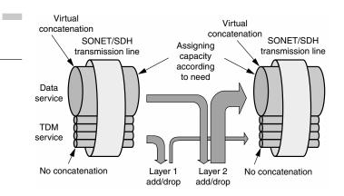
**Figure 16-3** Layer <sup>1</sup>/<sub>2</sub> hybrid add/drop.
