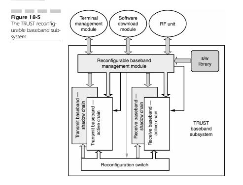
*Reconfiguration switch.* A typical on/off switch. It implements the on/off signal from the RMM in order to switch the shadow chain on and the active chain off.<sup>1</sup>
