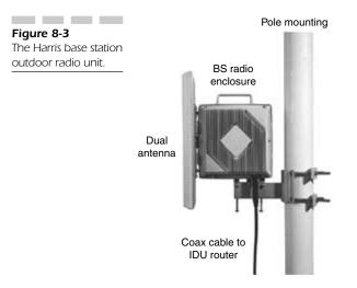
a pole, a tower, or a wall. The remote station ODU is an unprotected unit, where a single transceiver with a medium-power amplifier is used. The enclosure is directly connected to the flat-panel antenna. In addition, an alignment indication connector is also provided for antenna installation and alignment with the base station.
