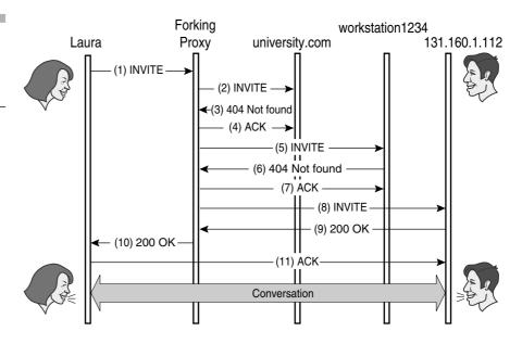
**Successful Final Responses** Successful final responses are transmitted reliably end to end between UAs and do not need the hop-by-hop mechanism used by other final responses (Figure 5-27). Only the UA that originated an INVITE can send an ACK for a final successful response. Therefore, regardless of the transport protocol used (reliable or unreliable), a UA retransmits successful final responses until it receives an ACK from the originating UA.
