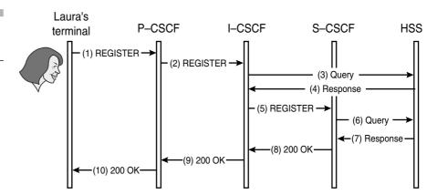
be, to the P-CSCF. The P-CSCF is the point of contact between the terminal and the network. The P-CSCF sends the REGISTER to the I-CSCF. The I-CSCF has to choose an S-CSCF for the user. To do that, the I-CSCF consults the HSS. Note that the protocol used between them is not SIP. The HSS can be thought of as a location server. It interacts with SIP entities, but does not speak SIP.
