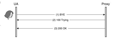
to ensure that the UA also receives it. The UA retransmits the request until the proxy proffers a final response. The proxy retransmits its final response as long as it continues receiving request retransmissions. When retransmissions stop, the proxy determines that the UA has received the final response (Figure 5-31).
