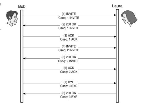
**Cseq in ACK** An ACK request has the same Cseq as the INVITE it acknowledges. This enables proxies to generate ACKs for non-successful final responses without creating new Cseqs. In fact, new Cseqs can only be created by the UA, which ensures that Cseqs are unique.
