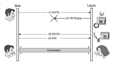
Figure 6-4 The PRACK ensures that the provisional response is transmitted reliably.
