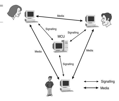
description to each participant with the multicast address that will be used. In the case of unicast, the conference unit adds a new m line though a re-INVITE every time a new participant joins the conference to trigger all current users to send media to the new participant as well.
