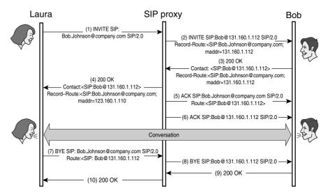
UA receives the INVITE complete with this Record-Route header and includes it in the 200 OK response. Bob's UA also adds its Contact header to the response.
