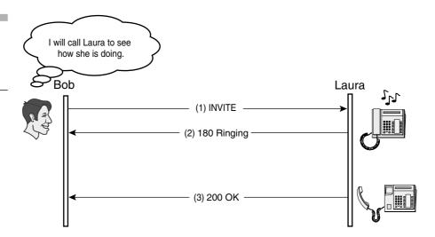
**ACK** ACK requests are used to acknowledge the reception of a final response to an INVITE. Thus, a client originating an INVITE request issues an ACK request when it receives a final response for the INVITE, providing a three-way handshake: INVITE-final response-ACK (Figure 5-2).
