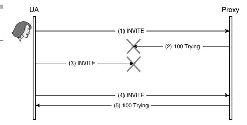
**Transmitting Responses to an INVITE** We have seen that provisional responses are used to prevent hop-by-hop INVITE retransmissions. However, nothing ensures that a provisional response from the callee's UA will reach the caller's UA. Proxies in the path will usually forward the response to the previous hop once, but will not retransmit if it fails to arrive (Figure 5-24).
