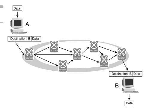
Packet headers on the path incorporate the virtual-circuit identifier that was assigned previously, and routers forward packets accordingly.
