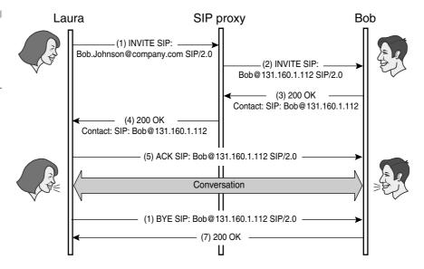
**Cseq** The *Command Sequence* (Cseq) header has two fields: an integer and a method name. The numerical part of the Cseq is used to order different requests within the same session (defined by a particular Call-ID). It is also used to match requests against responses. For instance, Bob sends an INVITE to Laura with the following Cseq:
