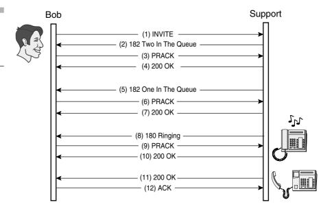
Making PRACK into a request-response transaction enables proxy servers that are not PRACK aware to route this new method properly. If PRACKs had no response, proxies would have to learn a new method in order to apply special routing that doesn't wait for a response.
