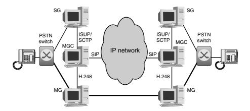
In SIP bridging scenarios, neither PSTN end user is willing to lose any special feature provided by the PSTN just because the call is traversing a SIP network. Therefore, SIP bridging has to provide a certain level of feature transparency. The information contained in the PSTN signalling messages has to be preserved when converted to SIP messages in the IP network, so that the egress gateway can regenerate the PSTN messages properly at the remote-user terminal.
