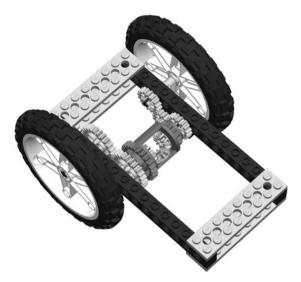
Fig. 9-27. Differential to measure turn angle.
