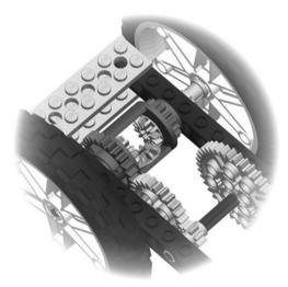
Fig. 9-26. Differential power transmission.
