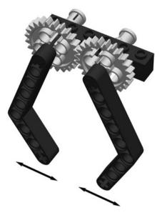
Fig. 14-8. Two-link synchronized gripper.
