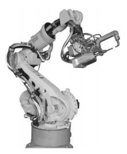
Fig. 1-2. Arm with welding attachment (photo courtesy Motoman).
