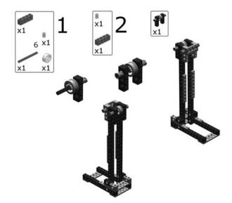
Fig. 3-16. Single pulley.
