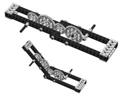
Fig. 9-14. Gears around a corner.
