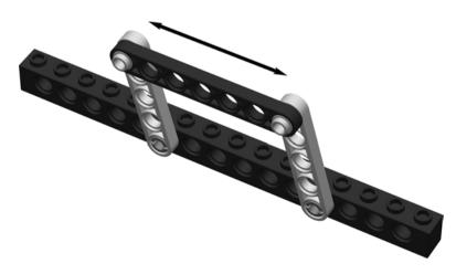
Fig. 14-10. Four-bar parallel motion.
