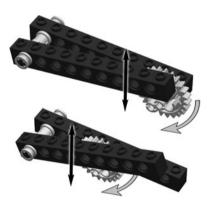
Fig. 14-5. Cam and levers for continuous motion.
