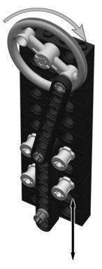
Fig. 14-7. Better rotary to reciprocal motion.
