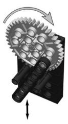
Fig. 14-3. Rotary to reciprocal motion.
