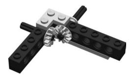
Fig. 9-18. Bevel gear.
