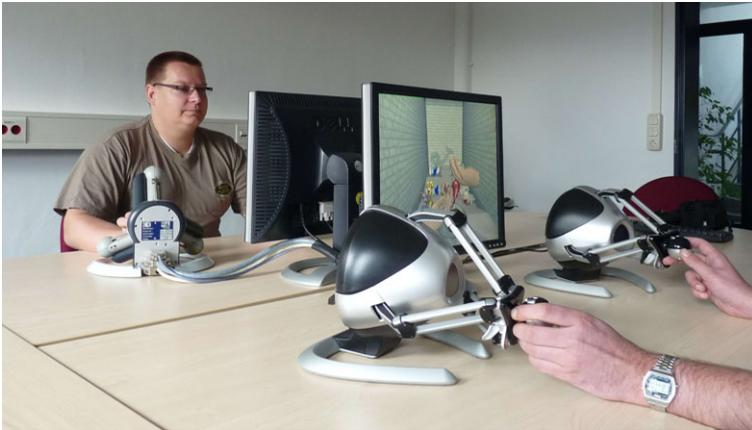
**Fig. 7.17** The two-player setup with four haptic devices for our user study
