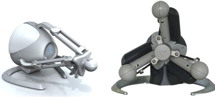
**Fig. 7.19** The haptic devices that we used in our evaluation: the 3 DOF Novint Falcon (*left*, courtesy of Novint Technologies Inc., USA) and the 6 DOF Haption Virtuose 6D Desktop (*right*, courtesy of Haption S.A., France)
