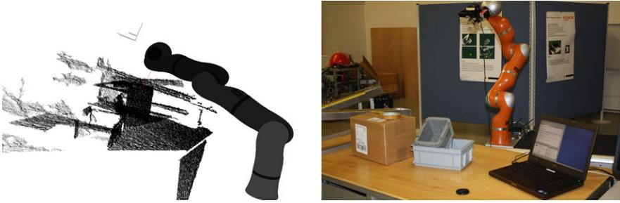
**Fig. 7.10** A typical point cloud recorded by the Kinect and the polygonal model of the LWR. The *red line* denotes the minimum distance between the LWR and the point cloud (*left*). The complete setup of our application is the KUKA Omnirob with a head mounted Kinect in front of a workspace (*right*)
