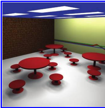
Figure 4.31. Analytic solution for soft shadows from two linear light sources per rectangle. Image courtesy of Poulin and Amanatides [465], ©Eurographics Association 1990. Reproduced by permission of the Eurographics Association.
