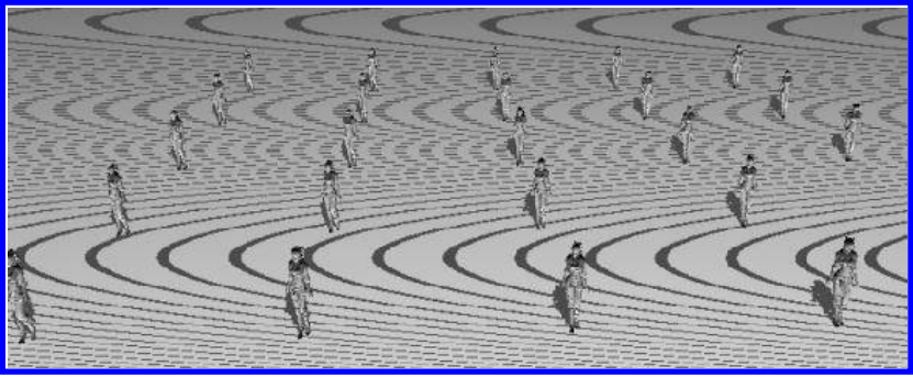
Figure 2.6. Moiré artifacts due to bad self-shadowing in shadow depth maps. Image courtesy of Bobby Anguelov ( http://takinginitiative.net ).
