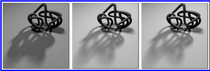
Figure 4.28. Comparing soft shadows from the following: penumbra wedges (left); the approach of Forest et al. (center); reference image (right). Image courtesy of Forest et al. [176]. Computer Graphics Forum ©2008 The Eurographics Association and Blackwell Publishing Ltd. Published by Blackwell Publishing, 9600 Garsington Road, Oxford OX4 2DQ, UK and 350 Main Street, Malden, MA 02148, USA. Reproduced by permission of the Eurographics Association and Blackwell Publishing Ltd.
