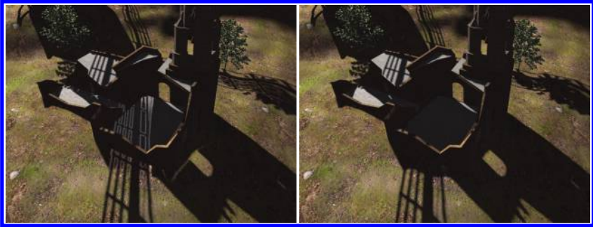
Figure 2.12. Light-leaking problem in the original variance shadow map implementation (left). Slicing into depth intervals reduces the light-leaking problems (right). Image courtesy of Lauritzen and McCool [334].
