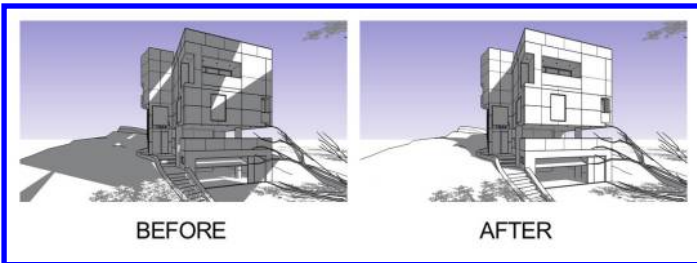
Figure 2.24. Shadow errors due to a single shadow count (left), with the correct shadows (right). Image posted by Aidan Chopra, courtesy of Google Sketchup and Phil Rader.
