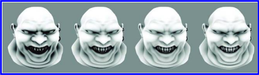
Figure 5.20. Multipasses of form-factor computations can reduce ambient occlusion over-occlusion. From left to right: one pass, two passes, three passes, and 200 random rays per vertex. Image courtesy of Bunnell [76], and model courtesy of Bay Raitt.
