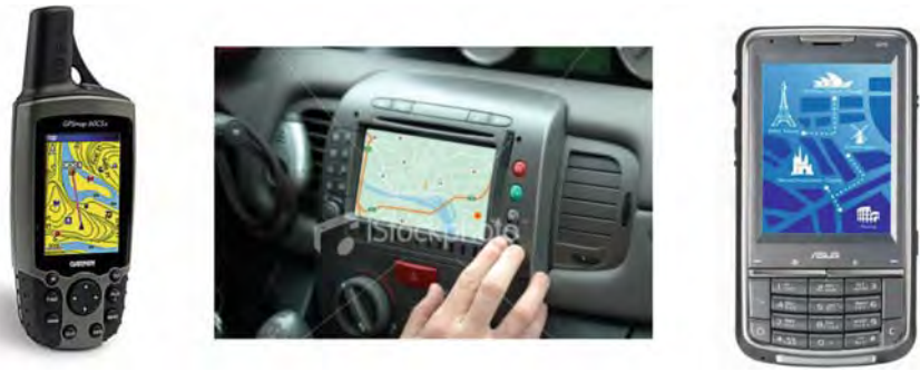
Fig. 7 Examples of GPS receivers: ( left ) handheld, ( middle ) automotive, and ( right ) mobile
