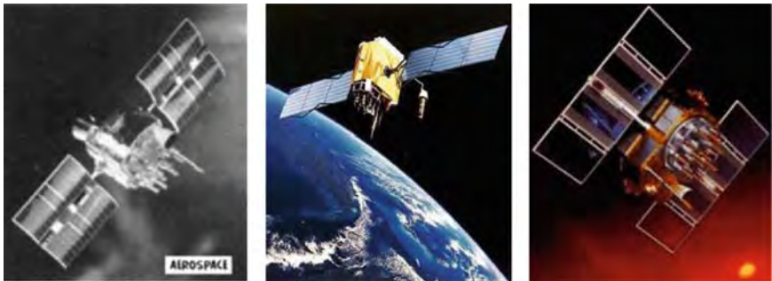
Fig. 5 GPS Block I, Block IIA, and Block IIF satellites
