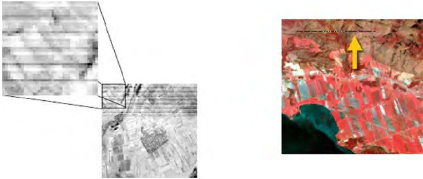
Fig. 23 (Left) Striping (or banding) error; (Right) line dropouts error
