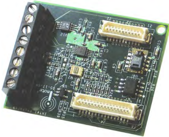
Fig. 2 Many commercial vendors are offering a variety of small, inexpensive wireless sensor platforms and sensor packages. This small platform from Crossbow Technology, Inc. contains an accelerometer, temperature, humidity, and light sensors – perhaps useful for environmental monitoring applications (Image courtesy of Crossbow Technology, Inc.)
