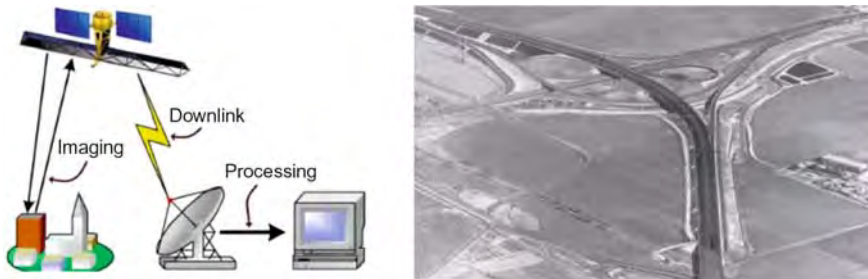
Fig. 19 (Left) Basic SAR image process; (right) example of images taken by a SAR
