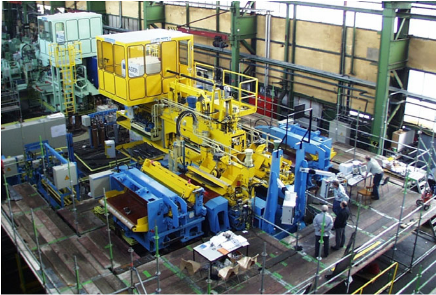
Fig. 1. Laser welding machine during testing and tuning process at Hugo Miebach GmbH., Dortmund, Germany
