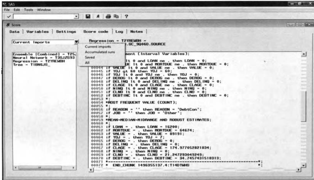
The Score code tab displays the internal SEMMA scored code from the Regression modeling node.
