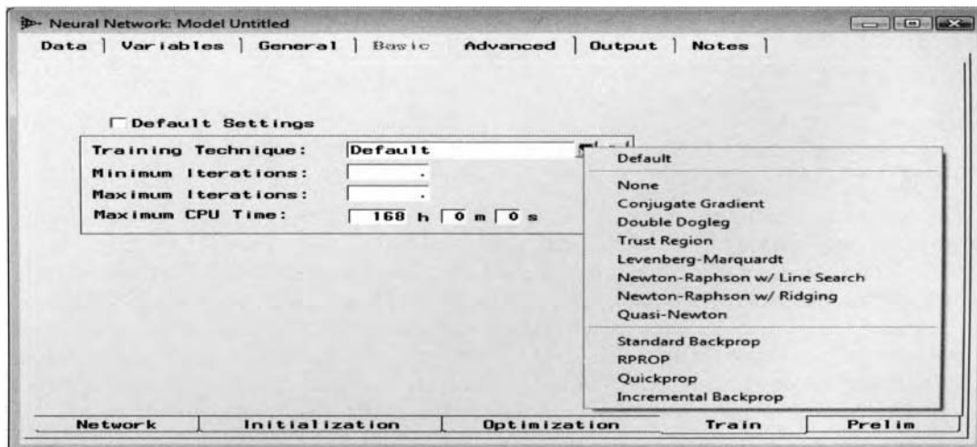
The Train subtab is used to specify the optimization method and configuration settings for network training.
