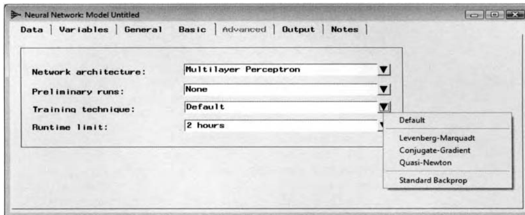
The Neural Network window is used to specify the optimization method for network training.
