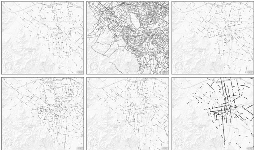
Fig. 6 Clustering result for rush hour after snow removal (2 days after the snowfall). The segments from the major roads are generally clustered together
