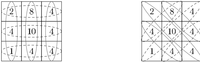
FIGURE 20.3: Representation used to mine JESs between classes of images. Strings are formed from horizontal, vertical, and diagonal sequences of symbols.
