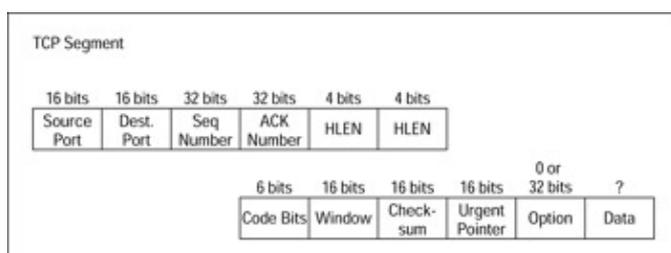
Figure 14-1: The format of the TCP segment.
