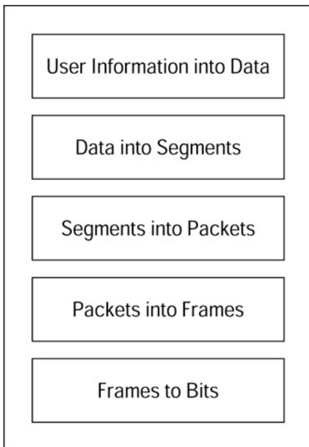
Figure 4-2: The five steps of data encapsulation.
