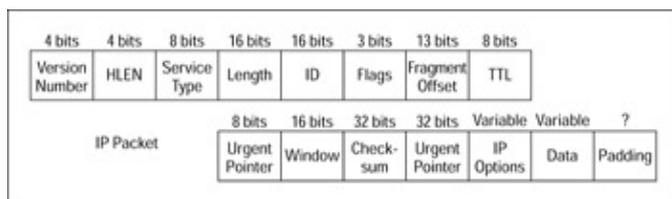
Figure 14–3: IP packet format.
