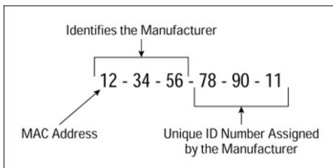
Figure 12-1: The MAC address and its parts.
