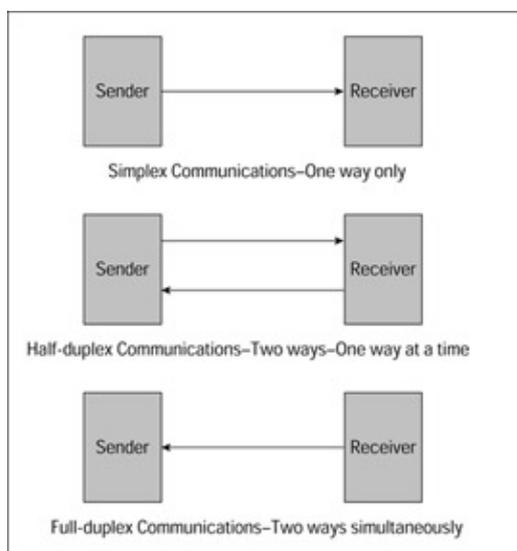
Figure 7–1: The three basic transmission modes.
