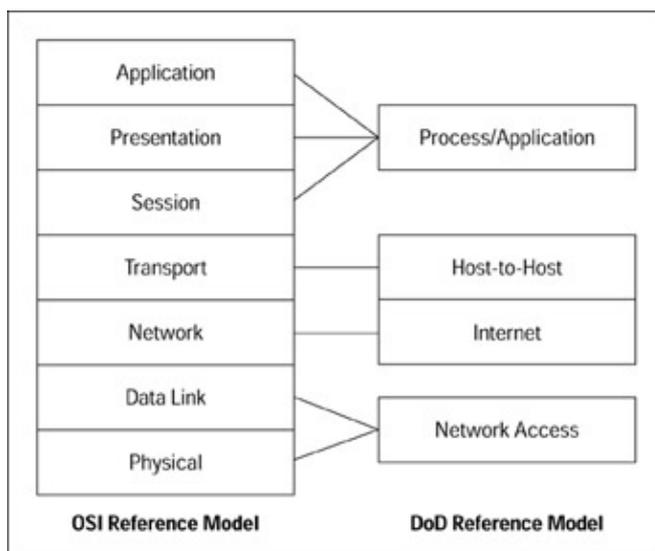
Figure 3-1: The seven-layer OSI model contrasts to the five-layer DoD model.
