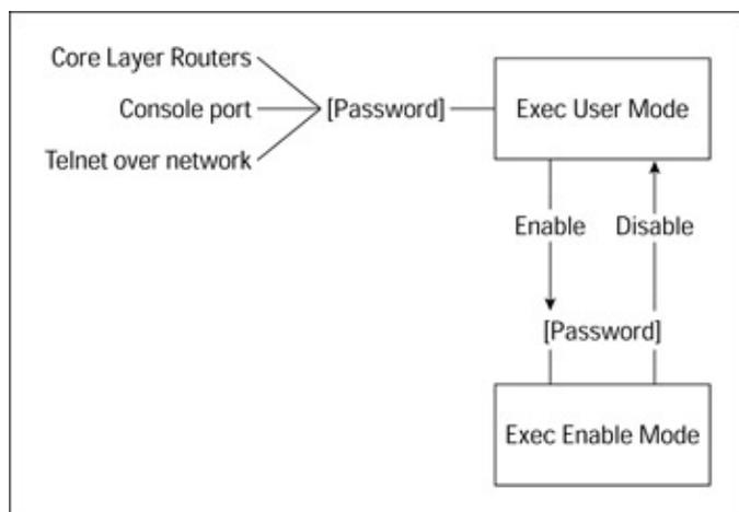
Figure 9–1: Logging into a router
