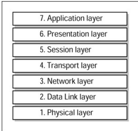
Figure 3–2: The layers of the OSI model.
