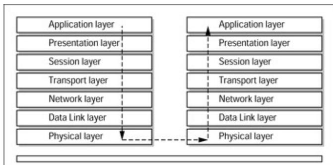
Figure 3-3: The route data takes through the OSI model's layers.
