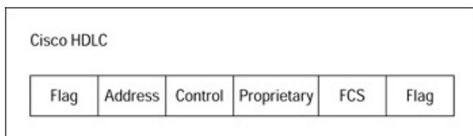
Figure 17-1: The HDLC frame format.
