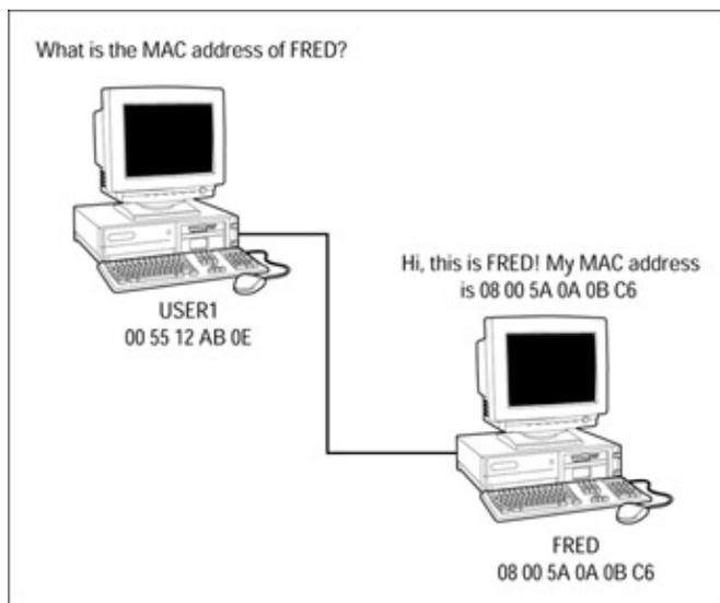
Figure 4–1: To resolve an unknown address on the network, a broadcast request is sent out.
