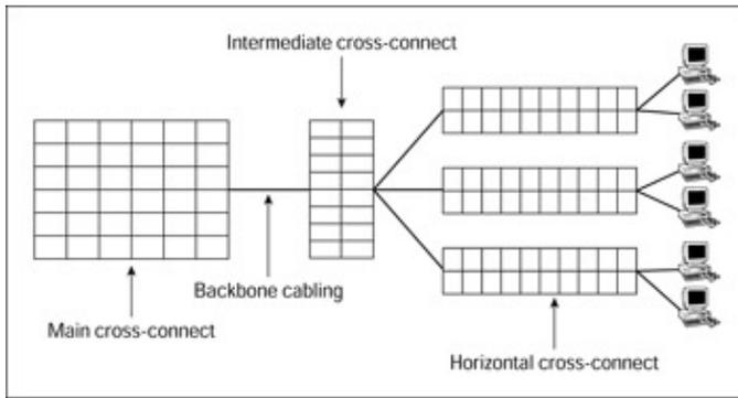
Figure 3–6: Backbone cabling provides the interconnection to the cross connects of a network.
