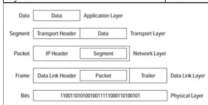
Figure 14-4: Five steps of data encapsulation.
