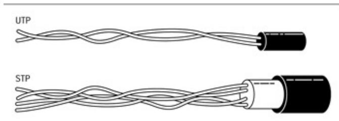
Figure 3-4: Twisted-pair wiring.
