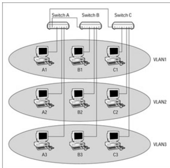
Figure 16–1: A VLAN workgroup created across three physical LAN segments.
