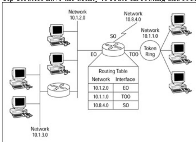
Figure 11-1: The routing table in a network router
