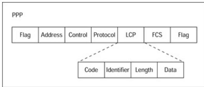
Figure 17–2: The PPP frame format.
