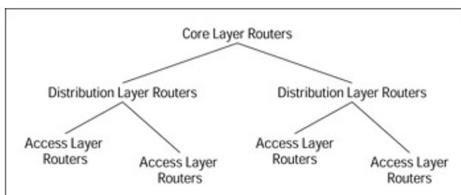
Figure 8-1: The layers of the Cisco router hierarchy.
