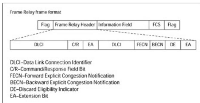
Figure 17-3: The Frame Relay frame format.
