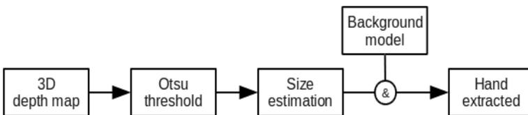
Figure 13.21: Flowchart of the hand extraction.
