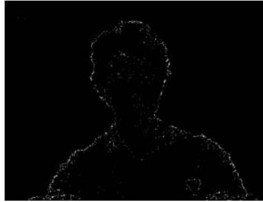
Figure 13.12: Image of a stationary subject after frame differencing and thresholding.
