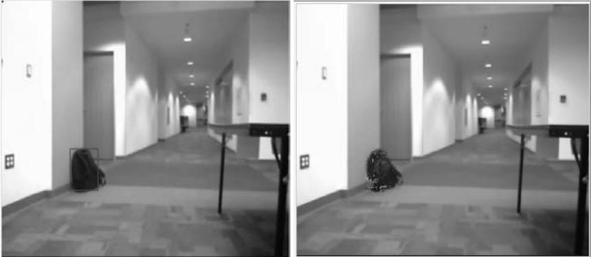
Figure 12.7: (a) Suspicious object detected and (b) modeled background.
