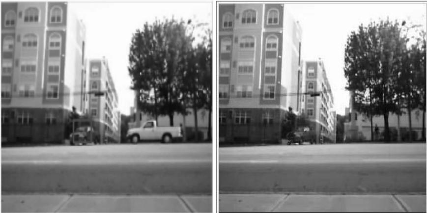
Figure 12.8: (a) Suspicious car detected and (b) modeled background.
