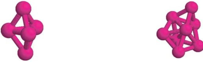
**Fig. 11.3** The stable structures of five and eight particles that interact with each other through the Lennard–Jones potential.
