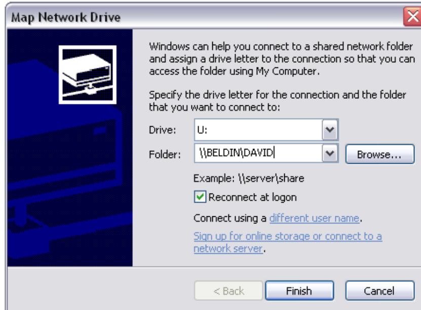
Figure 17.3 Dialog box for mapping a network drive.
